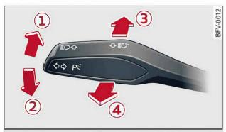
Fig. 38 Turn signal and main beam headlight lever
