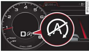
**Fig. 73** Instrument cluster: Engine stop temporarily unavailable
