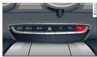
Fig. 108 Centre console: Button for park assist
