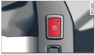
**Fig. 29** End face of (open) driver's door: Button for interior monitor/tow-away protection
