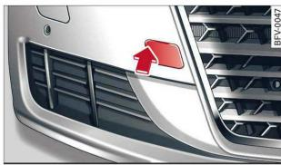
Fig. 242 Front bumper: Cover cap
