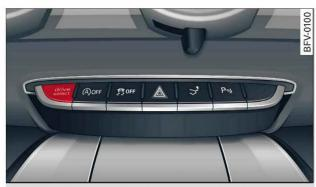
Fig. 96 Centre console: Button for drive select
