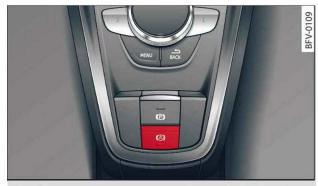
Fig. 76 Section of centre console: Button for hold assist
