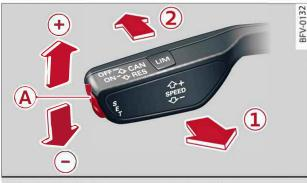
Fig. 86 Control lever for cruise control system
