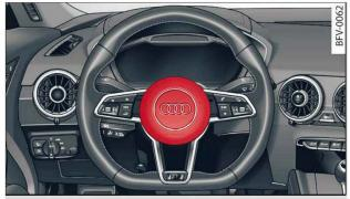
Fig. 200 Driver's airbag in steering wheel
