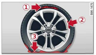
Fig. 227 Tyres: Irreparable tyre damage
