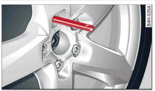
**Fig. 237** Wheel: Mounting pin in wheel bolt hole nearest to the top
