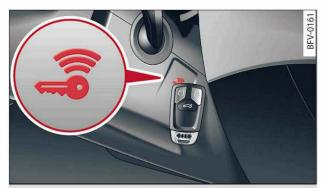
Fig. 71 Steering column/remote control key: Starting the engine after a malfunction
