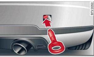
Fig. 245 Rear bumper: Fitting the towline anchorage\*
