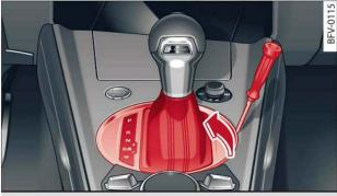
Fig. 82 Selector lever: Removing the cover
