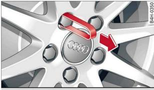
Fig. 231 Wheel: Wheel bolts with caps
