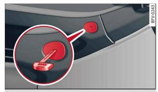
**Fig. 31** Accessing manual release lever on left of luggage compartment below rear window
