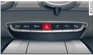
Fig. 40 Centre console: Switch for hazard warning lights
