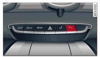
Fig. 99 Centre console: Button for parking aid
