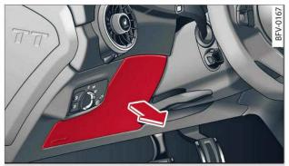
Fig. 246 Area near steering column on LHD vehicle: Cover
