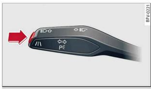
Fig. 89 Turn signal lever: Button for active lane assist
