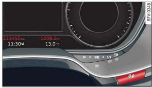
Fig. 11 Instrument cluster: Mileage recorder and reset button
