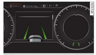
**Fig. 91** Instrument cluster: active lane assist switched on and in warning mode
