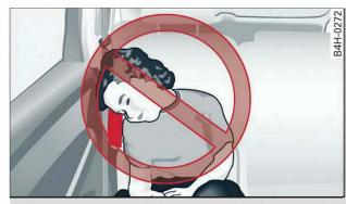
**Fig. 177** Illustration of a dangerous sitting position near the opening for the side airbag
