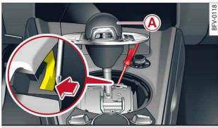
**Fig. 85** Manually releasing the selector lever from position P
