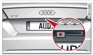
Fig. 103 Boot lid: Location of reversing camera
