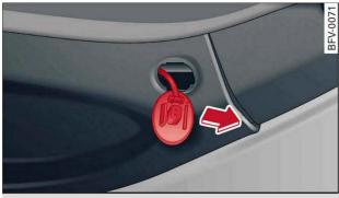
**Fig. 32** Manual release lever in luggage compartment (from inside)
