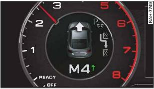
**Fig. 110** Instrument cluster: Prompt to keep driving forwards (a parking space has been detected)
