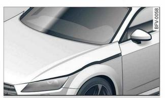
Fig. 185 Bonnet: Pedestrian protection system triggered
