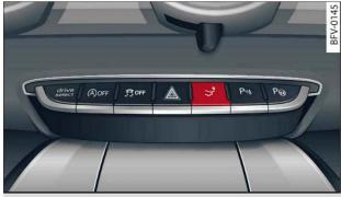
Fig. 114 Centre console: Button for rear spoiler
