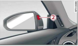
Fig. 93 Warning lamp on exterior mirror
