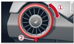
Fig. 67 Dashboard: Adjusting air outlet
