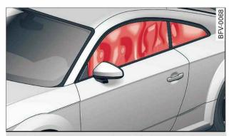
Fig. 207 Head-protection airbag in inflated condition
