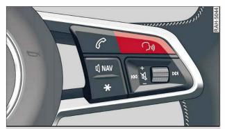
**Fig. 129** Talk button and right thumbwheel on multi-function steering wheel
