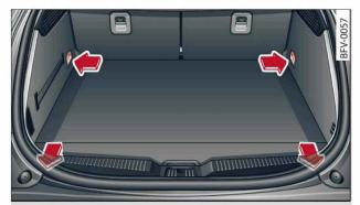
**Fig. 184** Location of fastening rings in luggage compartment
