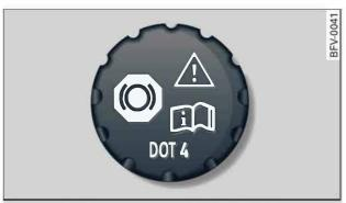
Fig. 219 Engine compartment: Cap of brake fluid reservoir
