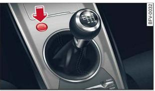
Fig. 70 Centre console: START ENGINE STOP button
