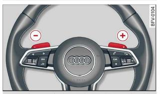
Fig. 81 Steering wheel: Manual gear selection with paddle levers\*
