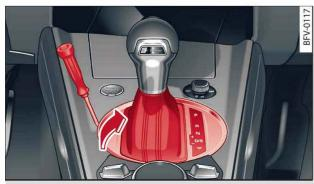
Fig. 84 Selector lever: Removing the cover
