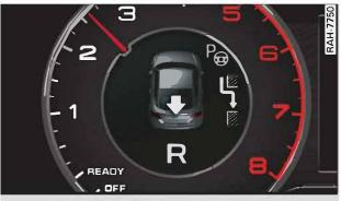
**Fig. 112** Instrument cluster: Manoeuvring into a parking space
