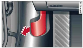
Fig. 213 Footwell on driver's side: Release lever
