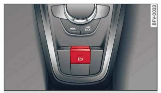
Fig. 75 Centre console: Parking brake
