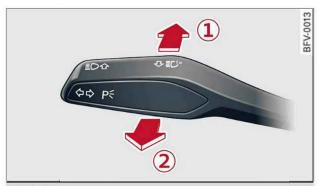
**Fig. 39** Turn signal and main beam lever: Switching main beam assist on/off
