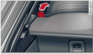
Fig. 62 Backrest release lever (left-hand side)
