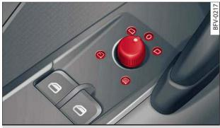
Fig. 43 Driver's door: Adjuster knob for exterior mirrors
