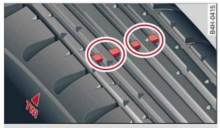
Fig. 222 Tyre tread: Tread wear indicators
