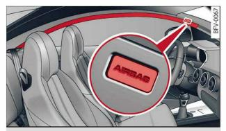
Fig. 206 Location of head-protection airbag above the door
