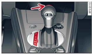
**Fig. 79** Detail of the centre console: Selector lever with interlock button
