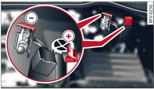
**Fig. 220** Engine compartment: Terminals for jump leads and battery charger
