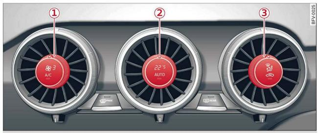
Fig. 66 Automatic air conditioner: Controls
