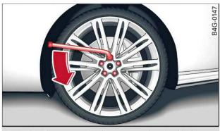
Fig. 233 Changing a wheel: Loosening the wheel bolts
