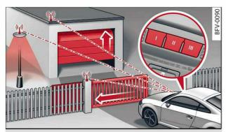
Fig. 34 Garage door opener: Examples of various devices which can be activated
