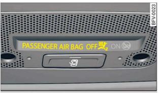
Fig. 199 Warning lamp lights up when passenger's airbag is deactivated
