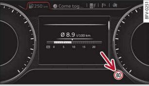
Fig. 15 Instrument cluster: Secondary display
