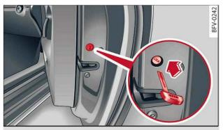
Fig. 28 Passenger's door: Locking manually
