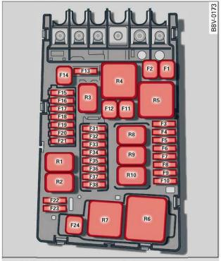
Fig. 250 Engine compartment: Fuse layout
