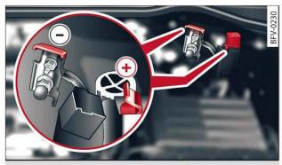
**Fig. 240** Engine compartment: Terminals for jump leads and battery charger
