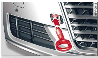
Fig. 243 Front bumper: Fitting the towline anchorage
