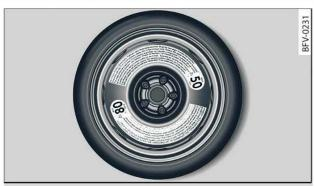
Fig. 239 Compact temporary spare wheel (example)
