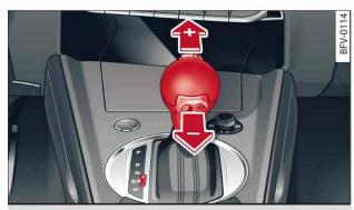
Fig. 80 Centre console: Manual gear selection using selector lever
