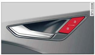
Fig. 26 Driver's door: Central locking switch
