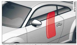
Fig. 205 Side airbag in inflated condition
