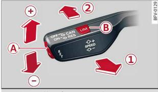
Fig. 88 Control lever for cruise control system
