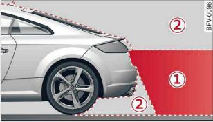
**Fig. 102** ①: Area covered by the reversing camera; ②: area NOT covered by the reversing camera
